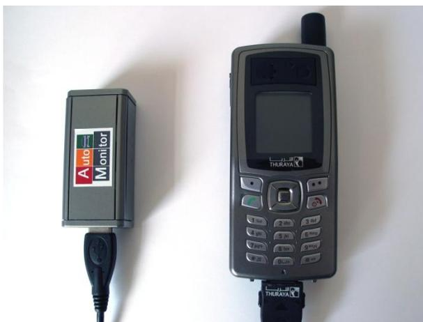
*World's smallest 3G router connected to the world's smallest satellite handset - Thuraya SO-2510*
