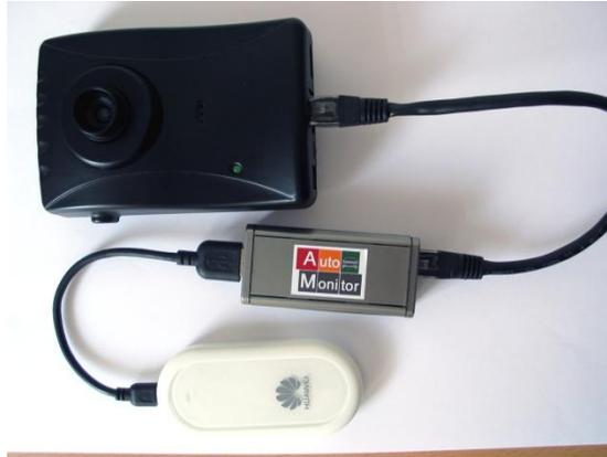
*AutoMonitor Jump connected to Huawei E220 3G modem and IP camera*
