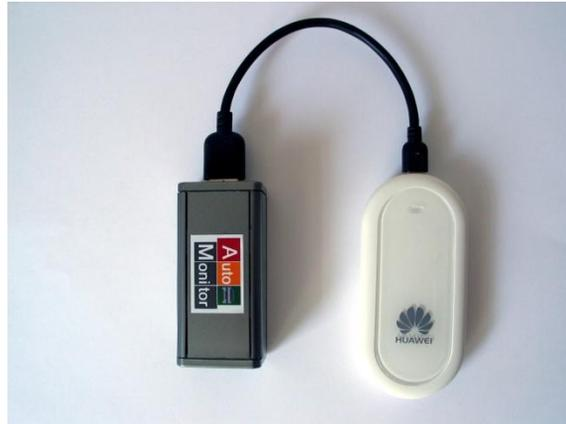
*AutoMonitor Jump connected to Huawei E220 3G modem.*
